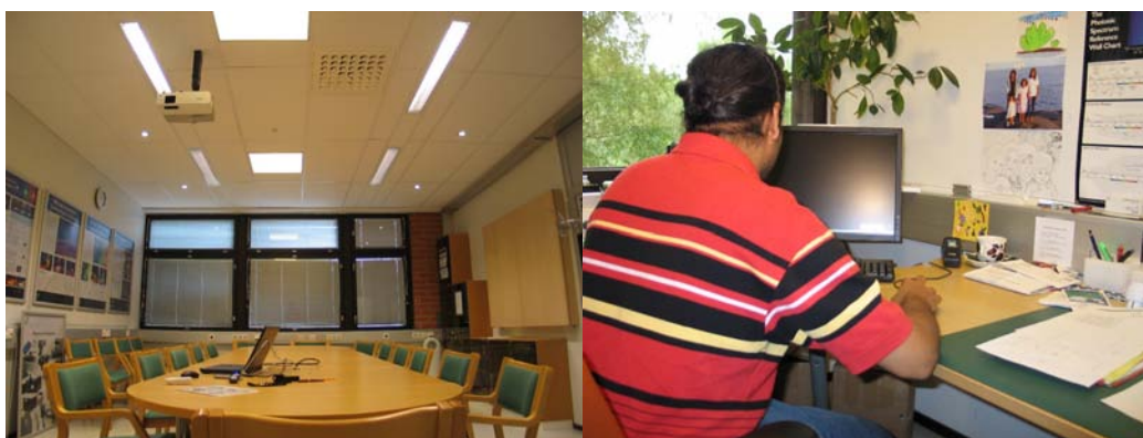
Figure 3-4. Luminaires and windows can induce direct glare, while light reflections from glossy surfaces and computer screens can induce indirect glare.
