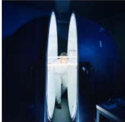
*Integrating sphere for luminous flux measurements.*
