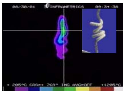
Fluorescent lamp electrode (small picture) and an infra-red image of the hot electrode.
