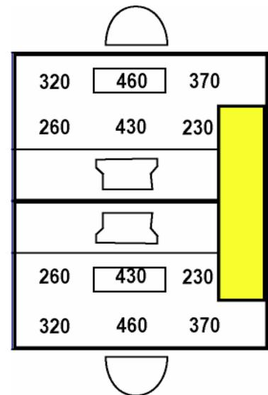
*Illuminance distribution on desk selected by the users for a direct-indirect lighting scheme shared by the occupants (2 x 54 W T5 dimmed at 65 %, power density 6 W/m<sup>2</sup>)*
