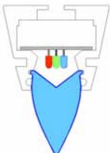
HESS 'Millennium' Aspheric lens mixing RGB-LEDs for street lighting application.
