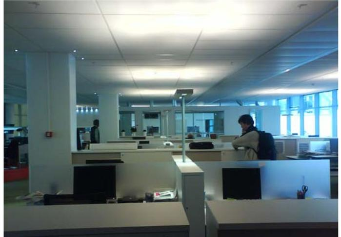
To use LEDs economically and with energy efficient solutions, T5 or CDM fixtures can not be replaced with LED fixtures 1 to 1. The conceptual thinking and planning methods must be quite different. E.g. for the workstations there is a combination with indirect lighting based on CDM 70 W and task lighting with LED 3 W. All other areas like conference and meeting rooms, corridors, communication areas and stairs are illuminated only with LEDs.
