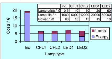
Lamp costs and energy costs of different lamp types with 2000 burning hours, electricity 15 c/kWh, interest rate 5 %, repayment period is lamp life divided by annual burning hours.
