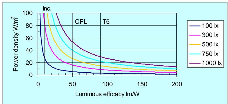
Power density ( $W/m^2$ ) as a function of luminous efficacy ( $lm/W$ ) on different illuminance levels (lx), maintenance factor was 0.75 and utilization factor 0.5.
